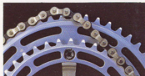
Rear side view of chain moving to low gear off W cut teeth.
