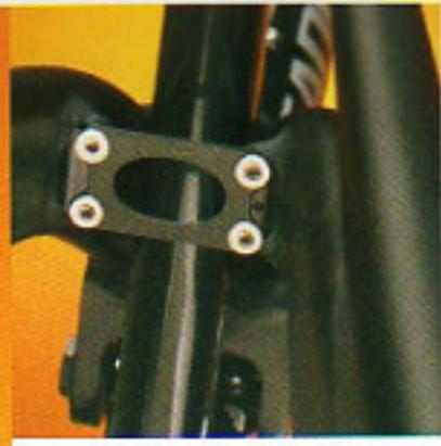
Superior handling and efficiency is all about lateral stiffness. The chain stay bridge boosts stiffness for superior tracking and power transfer.
