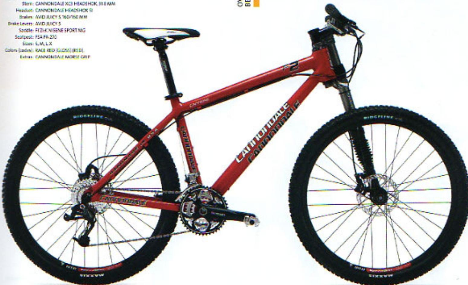
For 2008 we've oversized the seat stays of the Caffeine. By increasing the diameter of the tubes we've not only reduced wall thickness and shaved weight - but increased stiffness and power transfer.
