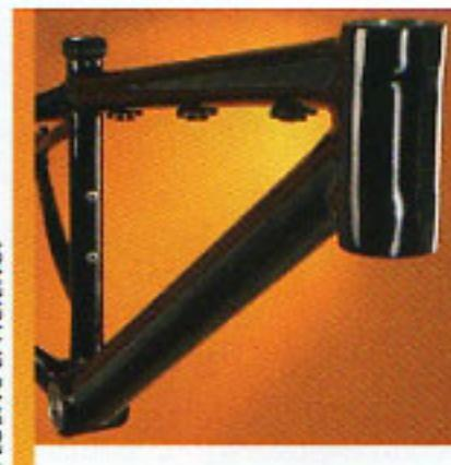
Each tube of the Taurine is optimized for a specific purpose. The down tube is oversized and round for maximum power transfer while the top tube is slightly ovalized for out-of-the-saddle sprints and climbs.
