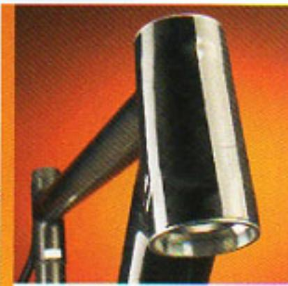
The head tube of the SuperSix is tapered to accept the shape of the tapered steerer which measures 1 1/8" at the headset and 1 5/8" at the fork crown. The result is superior handling and steering precision.
