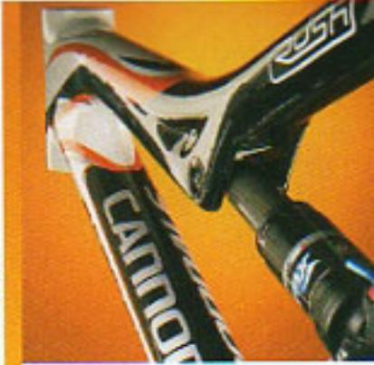
The full-carbon, monocoque front triangle is optimized for lightweight efficiency. Total bike weight is 33.7 lbs (10.8 kg). Longer hauls require less weight.
