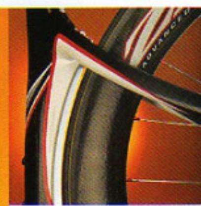
The Speed Shadow seat tube design hides the rear wheel from turbulent airflow.
