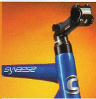
For 2008 the Synapse is equipped with a 2 cm removable head tube riser. This allows the rider to maintain a more upright, comfortable position. Remove it and flip the stem and you've got yourself a lightweight race bike.
