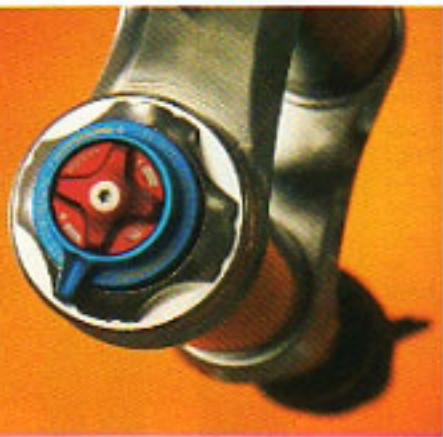
High-speed compression lockout and rebound adjust with easy access.
