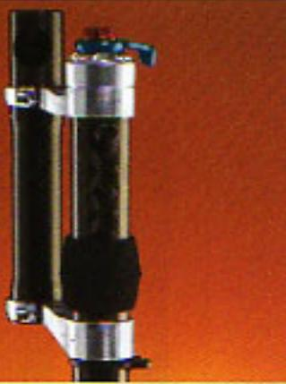
The Lightest gets lighter. Lightweight SL clamps are 30 grams lighter than our standard carbon clamps.
