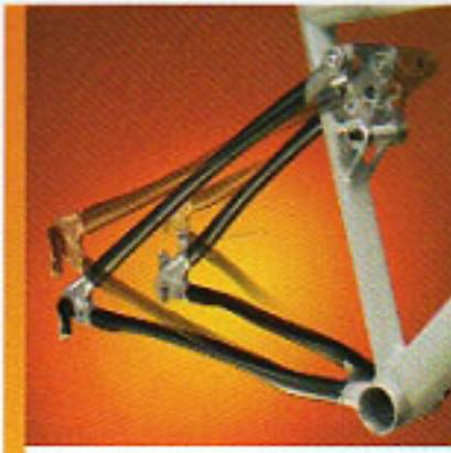
No hardware, bushings or contraptions. No bars, or bearings – just brains. The result is 100 mm of useful suspension. Carbon fiber optimized as the next generation of Living Hinge.
